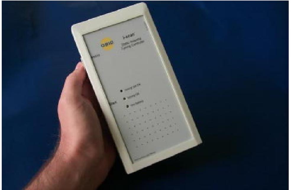
Control unit for antenna tuning of base and complementary antennas for the first setup of OBID® *i-scan* long-range applications or the adaption on changed surrounding conditions.
