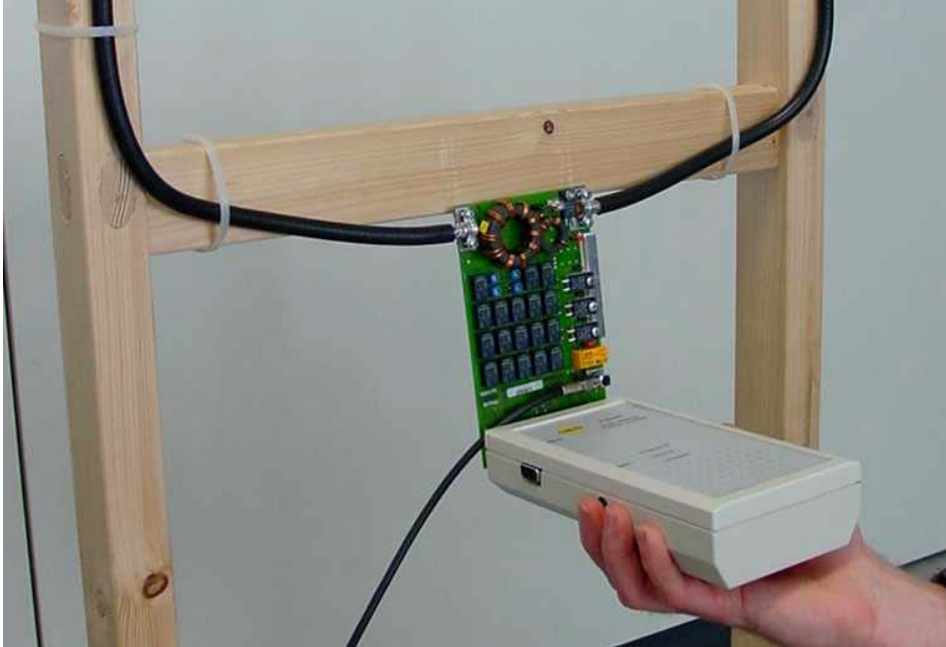
Figure 16: Tuning procedure at the base antenna
