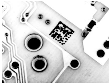
Figure 28 - Data Matrix Code Directly Marked on PCB Surface by Using Laser Etching Technology
