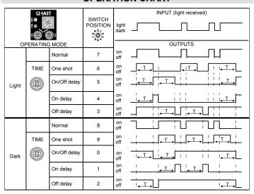
Note 1: Timing functions are selected by a rotary switch.
