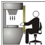
Fig. 7 Safety light curtain positioning
