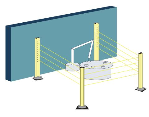
In applications where the monitoring of an area is required, safety light curtains can be used together with mirror for perimetral protection.
