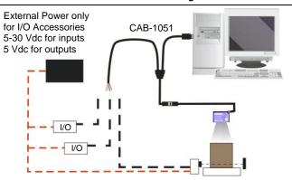
Serial + USB Models Using USB Port + I/O
