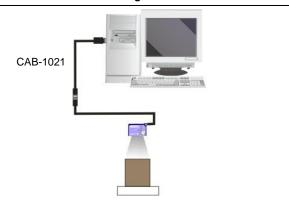
Serial + USB Models Using USB Port
