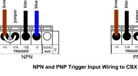
The electrical features of the two outputs at the CBX are the following:  $V_{CE} = 30 \text{ Vdc max}.$
