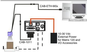
Ethernet + Serial Models Using Ethernet Interface
