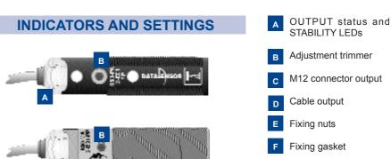
Single-turn trimmer for sensitivity adjustment. Rotate in a clockwise direction to increase the operating distance.
