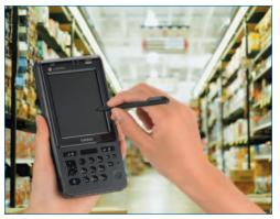
The built-in wireless LAN module (R- and CR-models only) enables safe high-speed and real-time communication in either the 802.11b or 802.11g standard with data transfer rates of up to 54 mbps. So an upcoming upgrade of existing WLAN networks will be no problem with using the IT-600.
