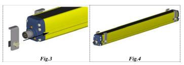
Insert the transparent plate and slide it along the binary under the fixing brackets. Once positioned correctly, tighten the screws with the N° 8 key, pressing the fixing bracket on the plate, until all the fixing brackets are blocked safely.
