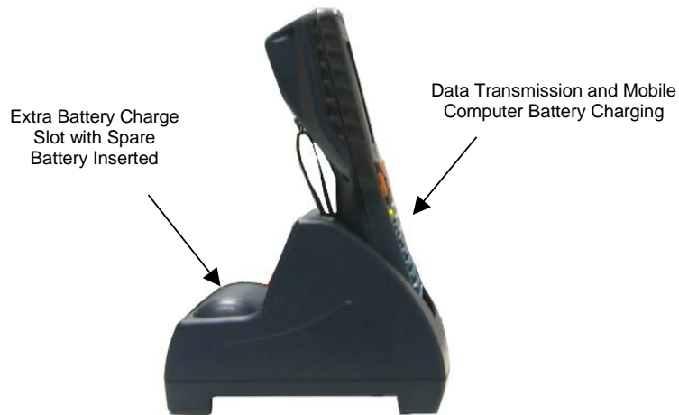
Figure 2 – Kyman-NET™ Single Cradle Desk Charging and Communication
