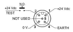
white = RESET/RESTART/RESTART MODE (\*) +24 Vdc 1 brown brown = +24Vdc **TEST** 2 = white = **EDM ENABLE** 3 = blue 0V = = 4 black **EARTH** = yellow = EDM = **NOT USED** 5 OSSD 1 grey
