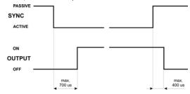
A typical application of the SYNC function is the necessity to detect a particular position in a multicoloured target while the other area must not be detected. This function can also be used to avoid erroneous detection during target-background transitions.
