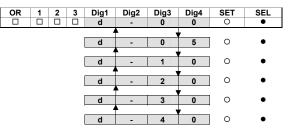
At each pressure of the SEL pushbutton, the different delay levels in ms are visualised in a cyclical manner at the output deactivation and moreover, the relative delay value will be stored When the "d-00" message is visualised the operating mode will be "run", and "rund" in all other cases.
