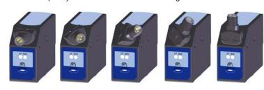
The operating distance is measured starting from the lens front face. The reading direction can be changed inverting the cap and lens. Mark detection on a reflective surface is improved adjusting the beam direction to 5° ... 20° from surface axis.
