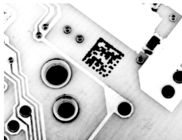
Figure 24 - DataMatrix Code Directly Marked on PCB Surface by Using Laser Etching Technology
