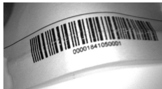
Figure 20 - Barcode Printed on Curved Surface Readable by Matrix 210™ in spite of Image Optical Distortion
