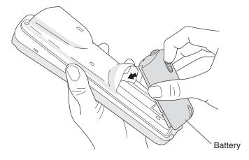
Insert the tabs on the bottom of the charged battery into the CK30 and snap the battery into place. The battery light on the CK30 blinks three times and the CK30
