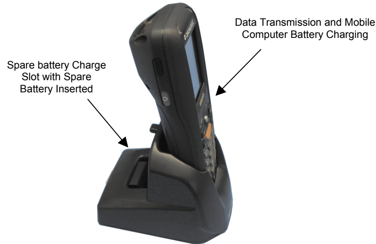
Figure 2 – Datalogic Memor™ Single Cradle Charging and Communication
