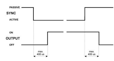
The SYNC wire is used also to determine the transmission direction when the RS485 serial connection
