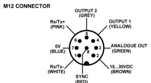
NOTE: the wire colours are referred to the cables manufactured according to the European
