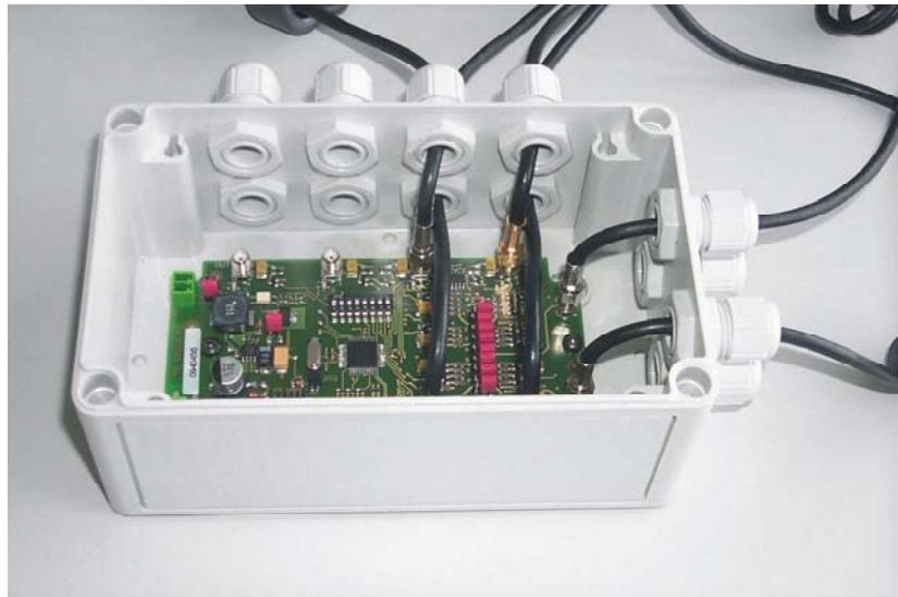
8 times Multiplexer for OBID i-scan® readers\* with external antenna connection for operation of several single- or gate antennas with only one reader.
